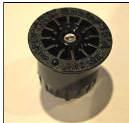
Using Cross-Sectional Scanning, Hunter Industries inspected the sprinkler nozzle to determine the cause of performance issues.
